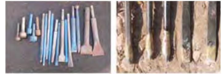
left: Assortment of tools for carving, moving, cushioning and installing carved limestone, Mason School (Lycee Professionel Jean Juares, Ile-de France).
