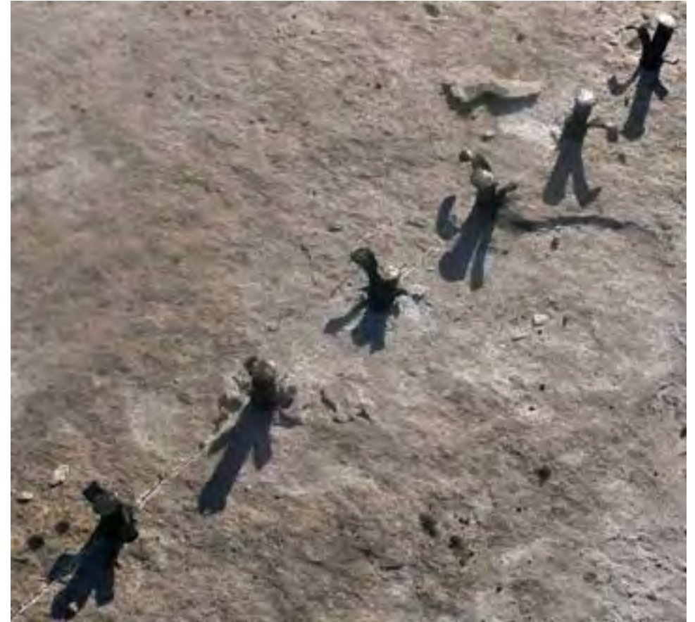
above: Splitting block stone with plugs and feathers in the Sadahali granite quarry, Peenya, India.
