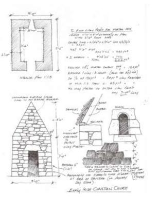
PROJECTS UNDERTAKEN AT STONEFEST X: A scale model of an early Irish church in stone with clay/sand/lime mortar; and the 'Krak,' a dry stone fortress with Turret Syndrome.
